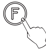
Light functions switch: press Once - colour rotation, twice - stop colour, three times - turn off lights.
